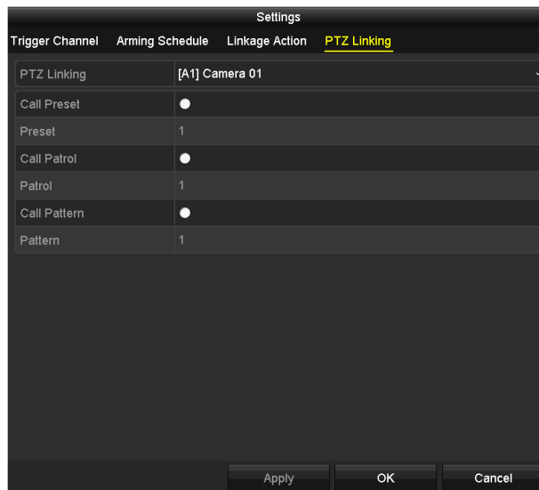
Figure 8-7 Set PTZ Linking of Alarm Input
