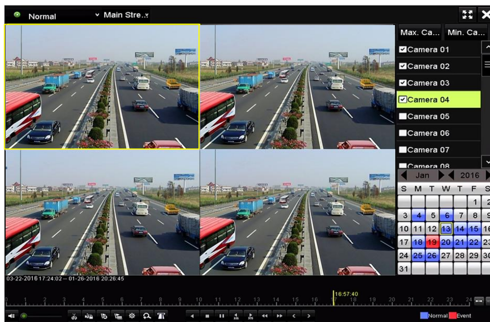
Figure 6-26 4-ch Synchronous Playback Interface
