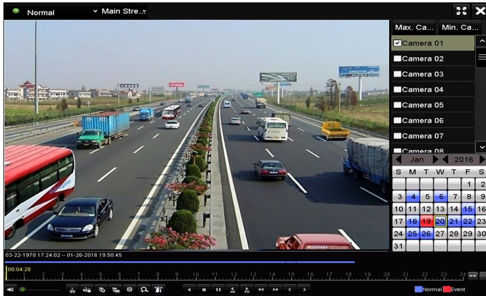
Figure 6-9 Interface of Playback by Time
