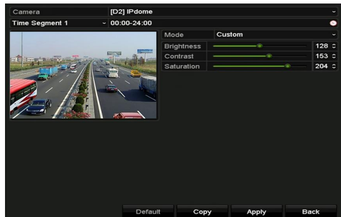
Figure 15-6 Image Settings Interface (IP Camera)
