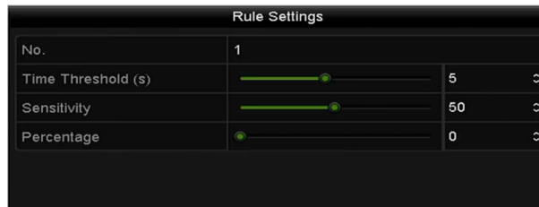
Figure 10-8 Set Intrusion Crossing Detection Rules
