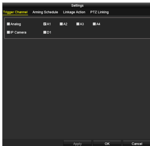
Figure 5-23 Set Triggered Camera of VCA Alarm
