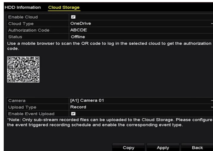
Figure 14-20 Upload to Cloud Storage Interface
